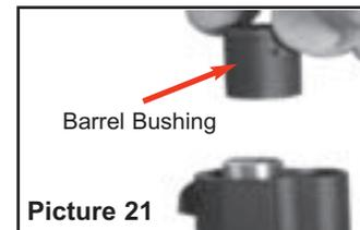
14. Turn the barrel bushing counterclockwise, push barrel and barrel bushing forward until barrel bushing lug is unlocked and barrel bushing can be removed from the barrel. See Picture 21.
