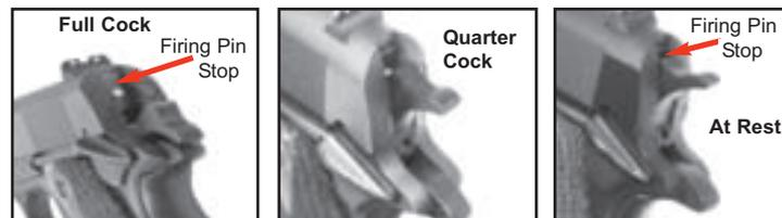
**AT REST**- this position is when the face of the hammer is resting on the firing pin stop.
